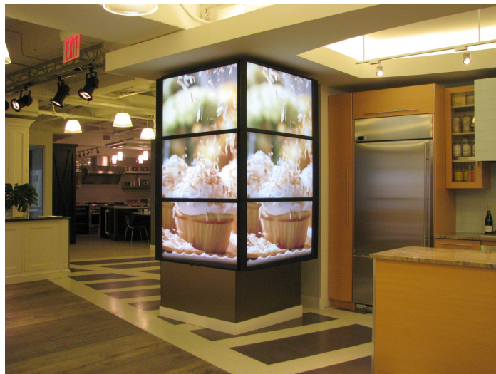
To achieve a Times Square-like visual effect, the GE Monogram Design Center used six NEC 46" MultiSync LCD4620 displays in a tile configuration. Installed in landscape orientation, these thin-bezel models are capable of displaying an overall portrait image in stunning clarity.
