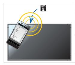
To read/write an adjustment value/setting value of the display, bring the terminal close to the Intelligent Wireless Data sensor of the display and press the READ / WRITE button of the application.
