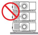
• Installation example when using 3 or more projectors The following installation is recommended when installing a combination of 3 or more projectors for multi-screen projection. [Installation example]
