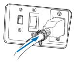
This completes the attachment of the power cable stopper.
