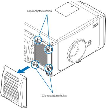
**<u>NOTE</u>** When removing the filter cover, remove it by applying force evenly. If you only apply force to one side, it may cause the clips to become damaged.
