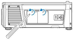
2. Grasp the standoff pillar of the screw securing the lamp cover and pull it up towards you to remove the lamp cover.
