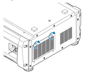
This completes replacing the rear air filter. Next, replace the side air filter.
