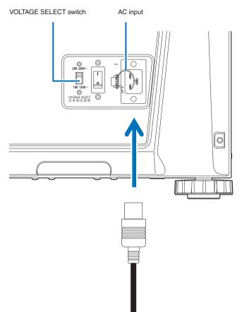
2 Set VOLTAGE SELECT switch according to the voltage being used.
