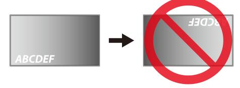
The monitor cannot be used when inclined  $16^\circ\,\text{or}$  more.
