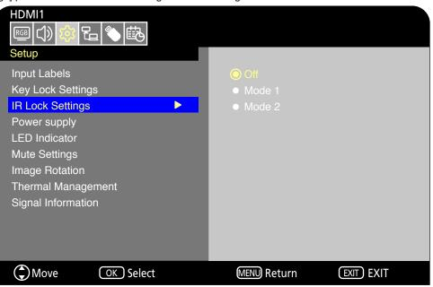
The [IR Lock Settings] prevent the monitor from being controlled using the remote control.
