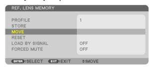
The lens will shift based on the adjusted values stored in the selected [PROFILE].
