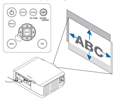
To set back the lens to the home position Press and hold the SHIFT/HOME POSITION button over 2 seconds. The lens mounted on the projector goes back to the home position. (roughly to the center position)
