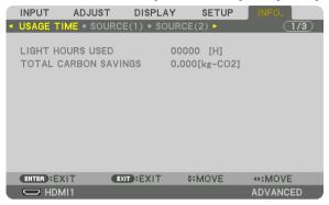
The [CARBON SAVINGS-SESSION] message shows the amount of CO<sub>2</sub> emission reduction between the time of changing to LIGHT MODE immediately after the time of power-on and the time of power-off. The [CARBON SAVINGS-SESSION] message will be displayed in the [POWER OFF/ ARE YOU SURE?] message at the time of power-off.
