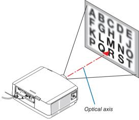
3. Press ▼ button to select the PERIPHERY on the onscreen menu, and then press either ◀ or ▶ button to align the focus of screen peripheral area. During this operation, the focus for around the optical axis will be maintained.
