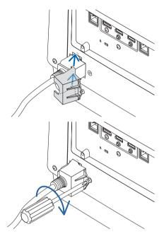
2. Fasten the screw on the power cord stopper.
