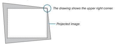
2. Pick up any one of the corners and align the corner of the image with a corner of the screen.
